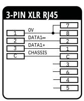
XLRJ45 adapter makes it possible to use any CAT-5 Ethernet cable as a DMX512 cable. XLRJ45 is available in four versions, 3-pin male or female XLR or 5-pin male or female XLR. The different adapters can be mixed to make for example a 5-pin to 3-pin cable. XLRJ45 is very useful for making a DMX512 cable quickly and at a very low cost.
