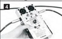
To test the cable's pin "1", twist the knob to position 1. If the indicating lights are green and yellow, your cable is testing successfully.
