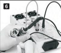
To use probe lines, insert two probe lines into the banana jacks. If you hear buzzing and a yellow LED light is on, it indicates that the line is testing successfully. To test audio cables with differing connectors, use the probe pen to connect them, if you hear buzzing it indicates the line is testing successfully.
