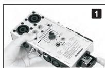
To install the battery, open the battery cover and insert into the cabin under "+" ".", push down until you hear a click which indicates the battery clocking.
