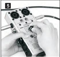
To test the cable's pin "2" and "3", twist the knob to position "2" and "3". If both LED lights are on, it indicates that pin 2 and pin 3 of this line is testing successfully. If one of the lights is not on, it is indicating there is a failure with this line.
