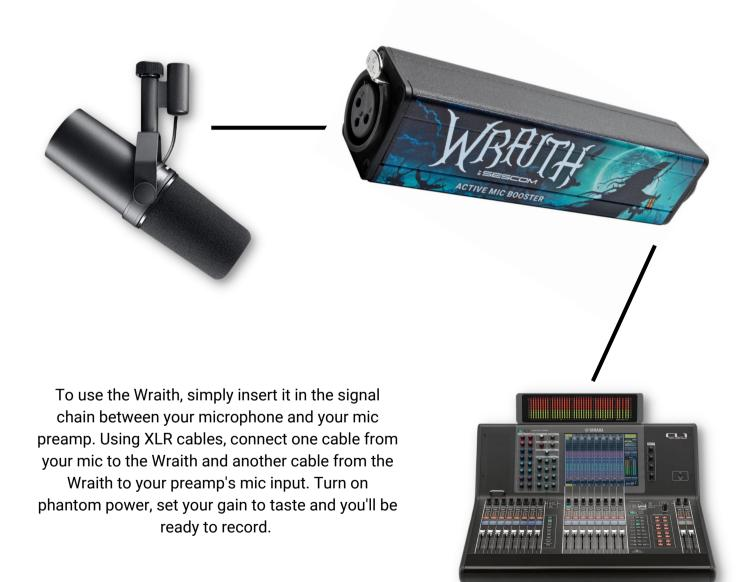
Please note that phantom power does not pass to the mic side of the Wraith, so your mic will not see the phantom power supply. If you want to use a condenser microphone with the Wraith, you will need an inline phantom power supply, like the Sescom SES-IL-PPI phantom power inserter.
